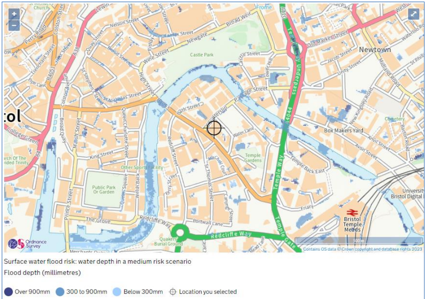
Figure 8: Medium Surface Water Flood Risk (Depth)
