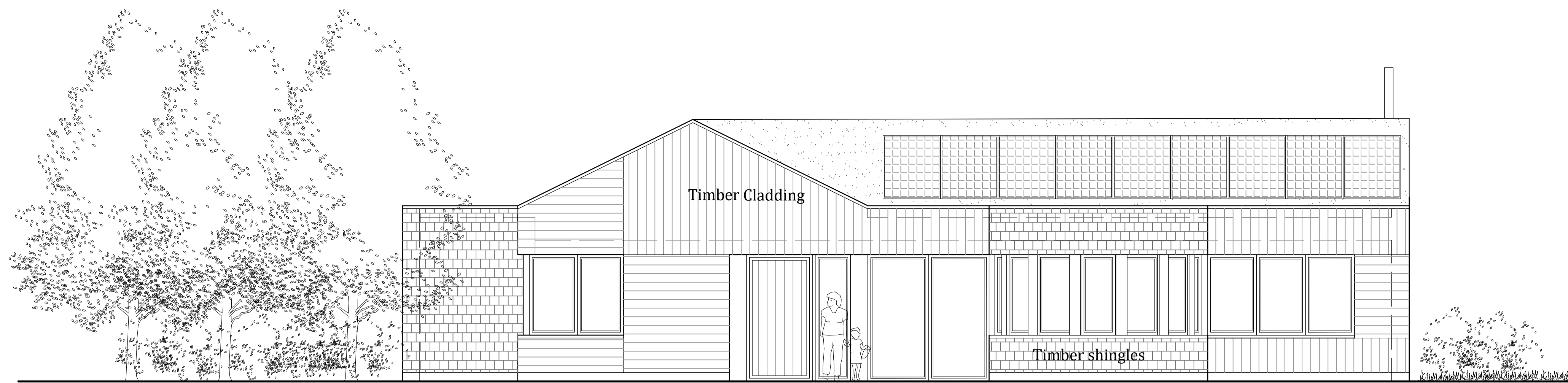
South West Elevation
