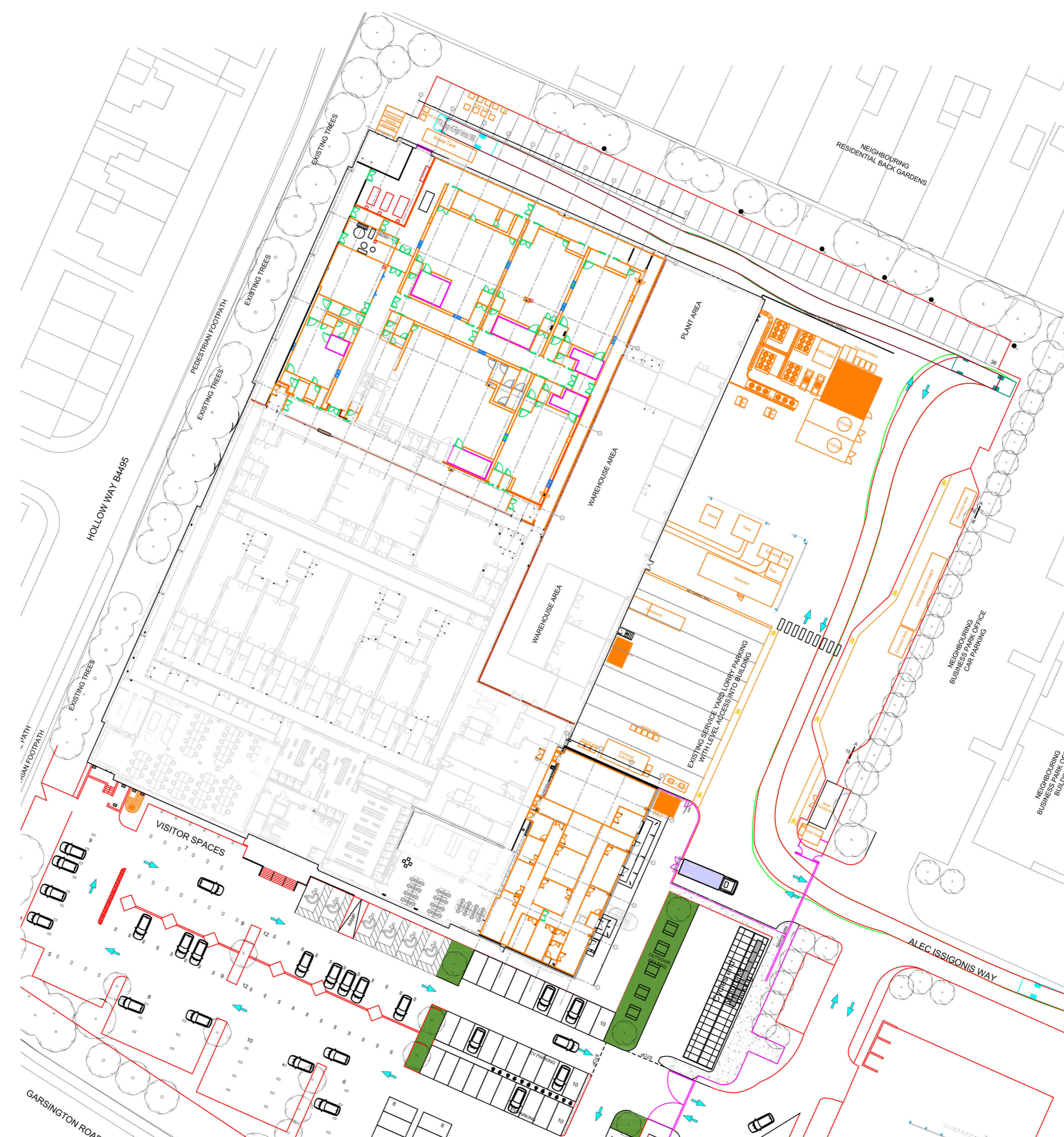
FTA Design HG Rigid Vehicle (Width 2.500m, length 10.000m) leaving site Note: Not enough room for turning vehicle would have to reverse out then turn
