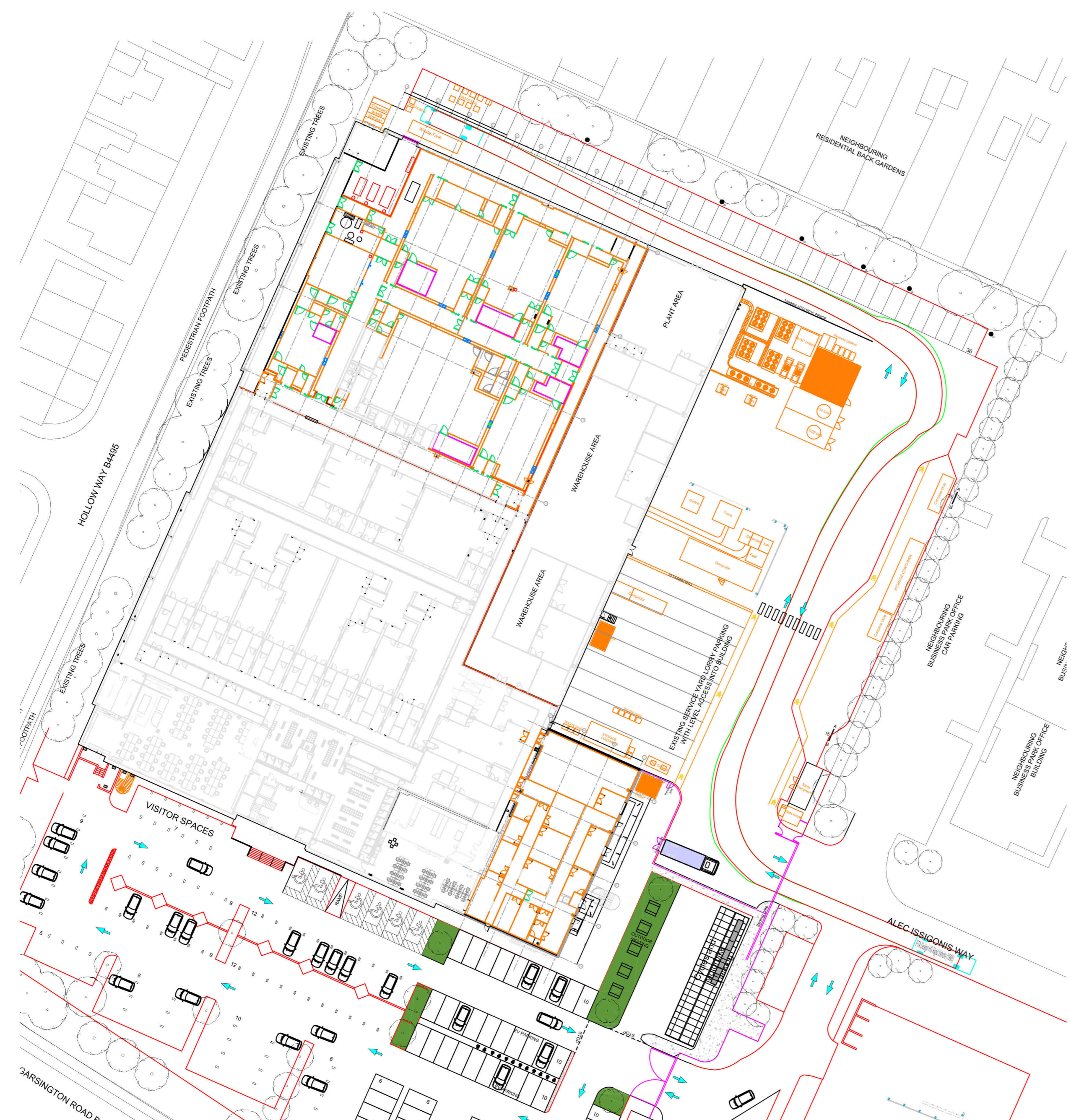
FTA Design HG Rigid Vehicle (Width 2.500m, length 10.000m) entering site (eg-Refuge collection/Waste tank)
