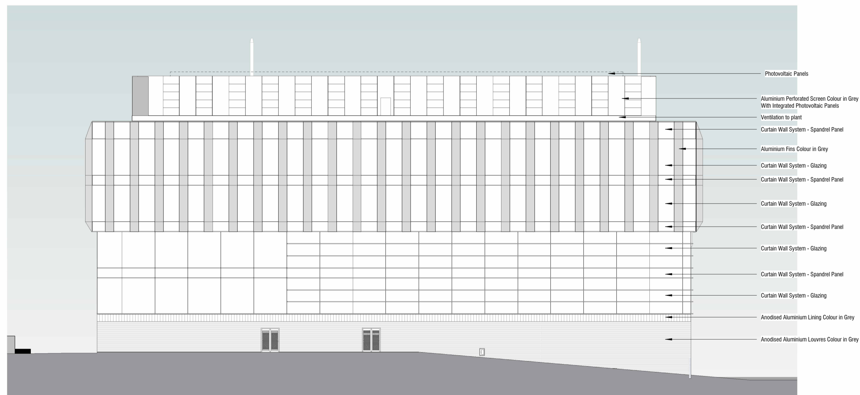
2 PROPOSED BUILDING 1 - NORTH WEST ELEVATION 1:200
