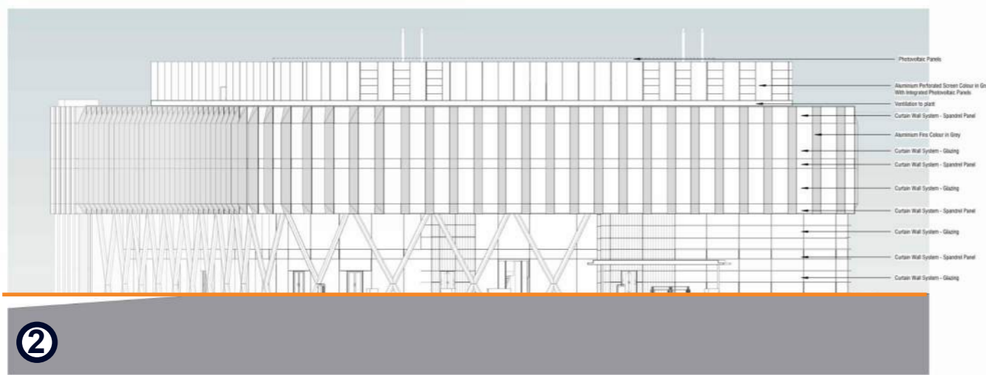
APPROVED BUILDING 3 NORTH WEST ELEVATION
