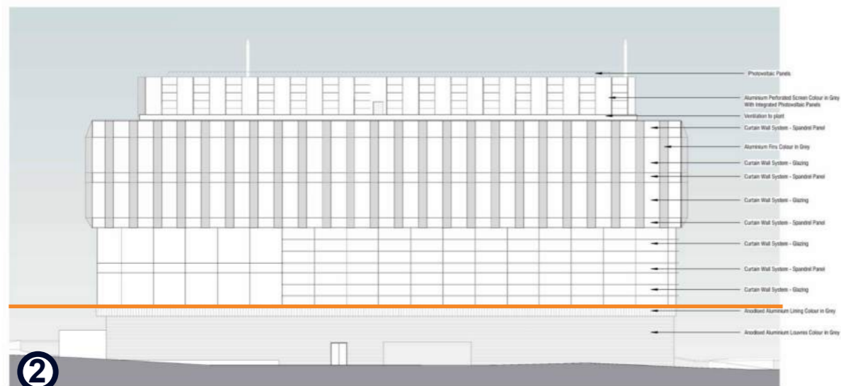
APPROVED BUILDING 1 NORTH WEST ELEVATION
