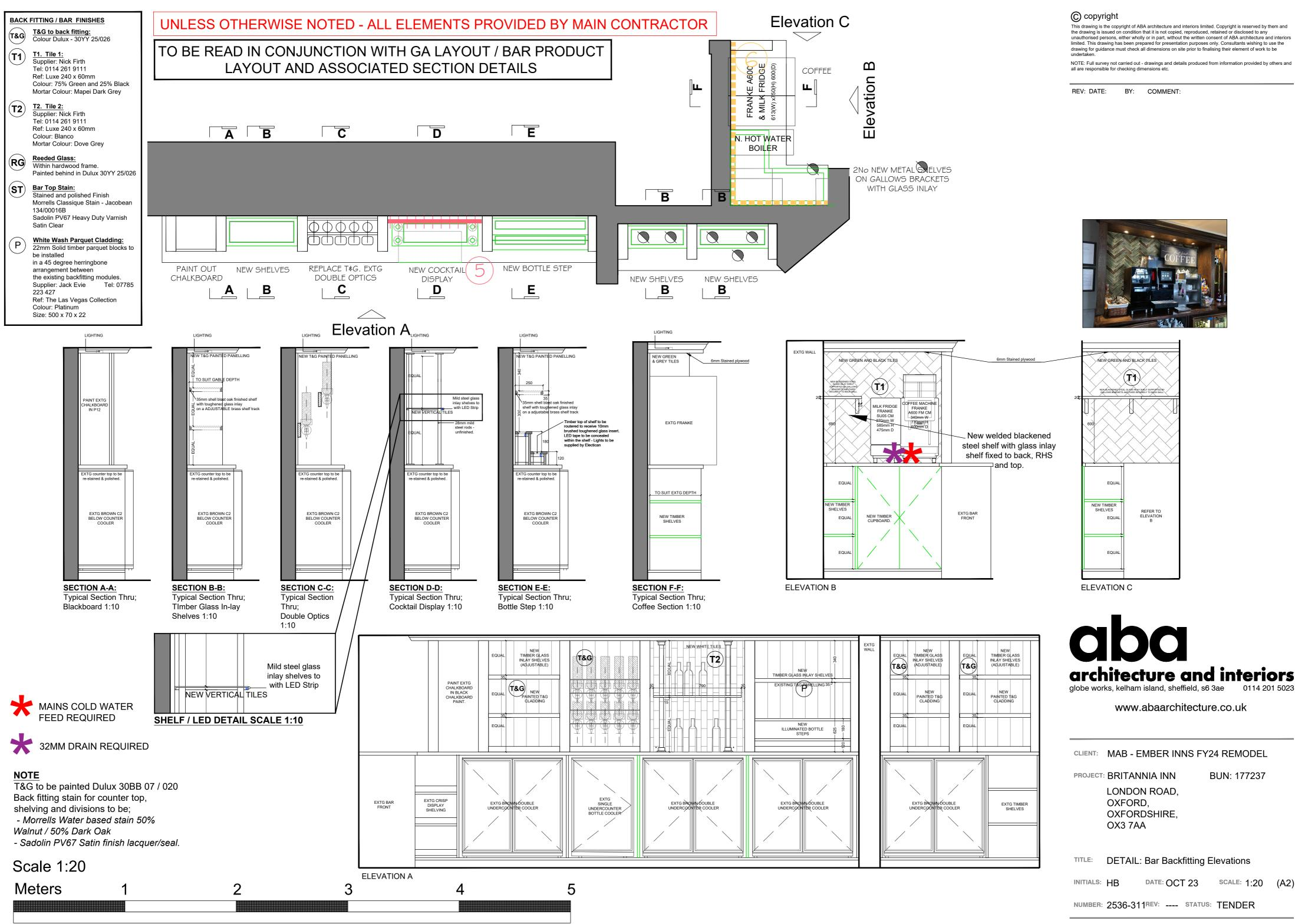
**DETAIL: Bar Backfitting Elevations**
