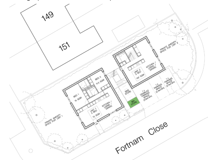
Fig. 111. Proposed site plan showing location of bin store within close proximity to the street to allow ease of access.
