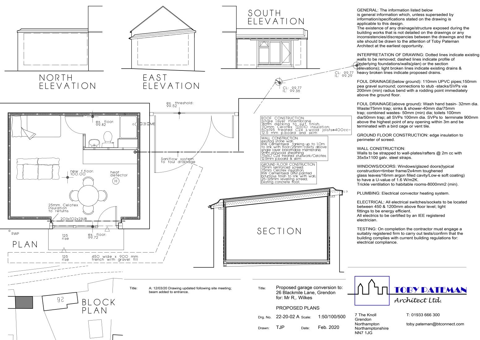
dia/50mm trap; all SVPs 100mm dia. SVPs to terminate 900mm
