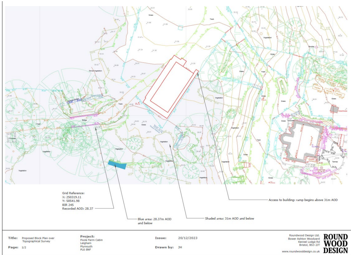
Fig. 11 Bir245 and Bridge 1D (approx. 20 – 30m upstream of Bir245) provide 2 flood levels 28.37m AOD and 31.0m AOD respectively. These are transposed onto the topo drawings for the Paddock Cabin (see fig. 11).
