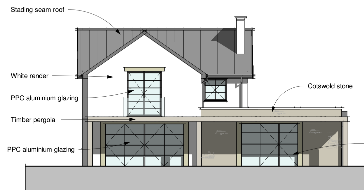
Proposed South Elevation 1 : 100@A1
