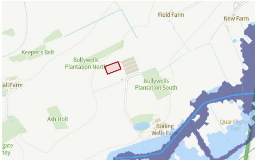
Extract from EA Flood Map depicting location of proposed units in Flood Zone 1 (clear). Flood Zone 2 is (light blue) and Flood Zone 3 is (dark blue).
