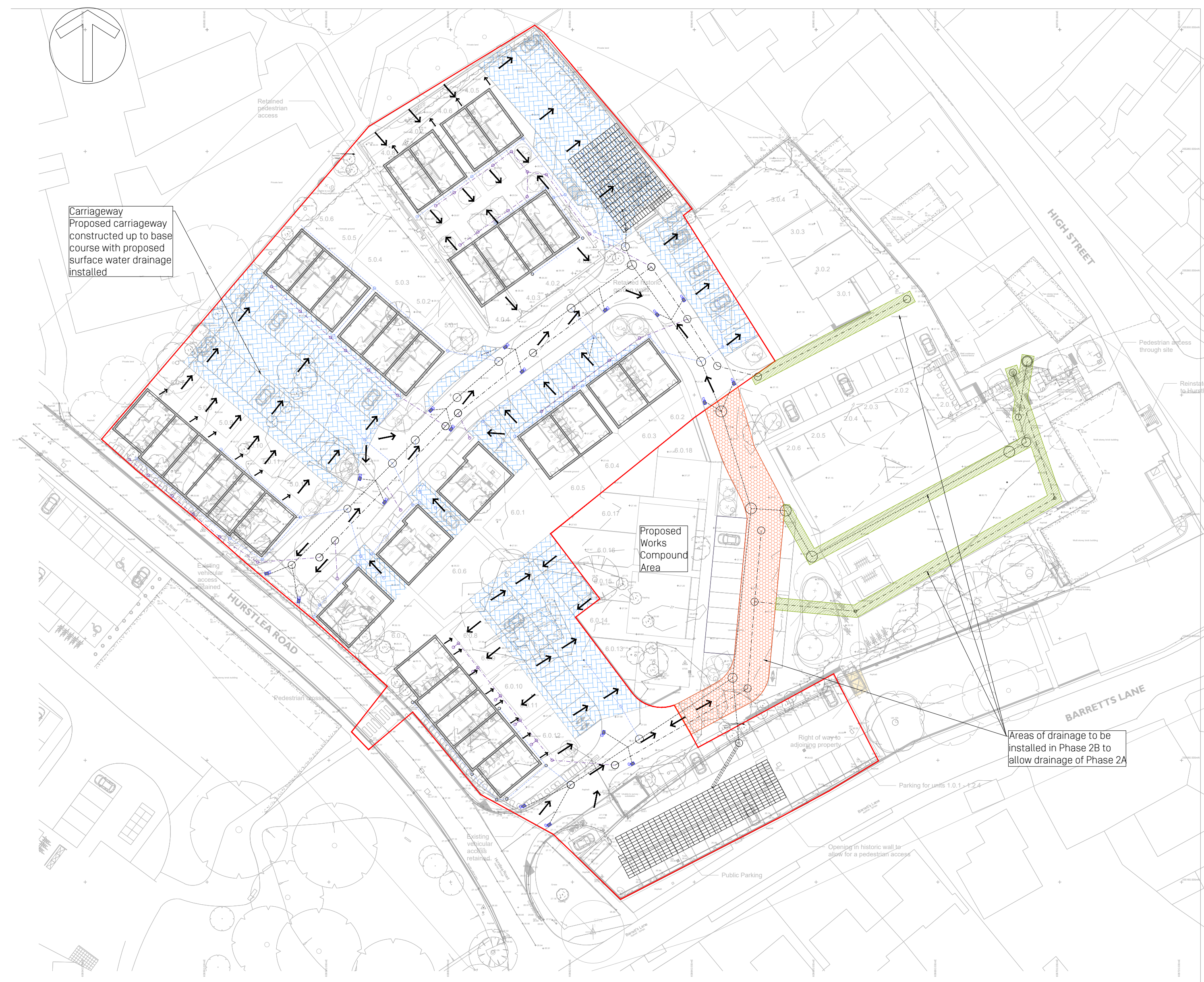
Phase 2 Drainage Construction Substructure & Shared Access Road
