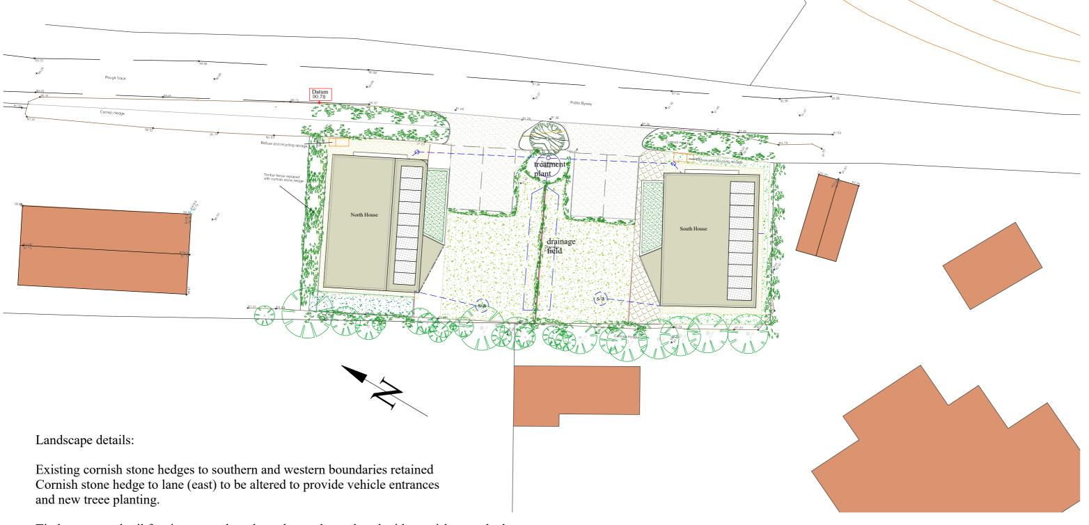
Timber post and rail fencing to northern boundary to be replaced with cornish stone hedge constructed in accordance with Bright Environment report ref: BE 548
