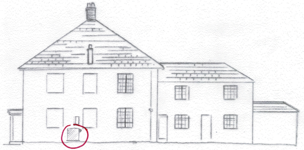
NORTH ELEVATION EXTERNAL BOILER CABINET
