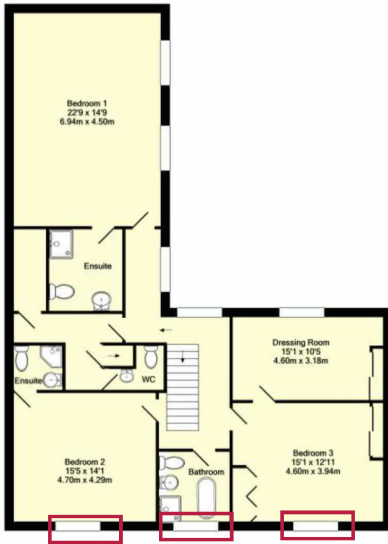
Figure 2 – Plan of First Floor showing location of 3 original sash windows to which the replacement windows on the Ground Floor would be matched (8 over 8 pane in Bedrooms 2 and 3 and 6 over 6 pane in Bathroom) [indicated by a red square]
