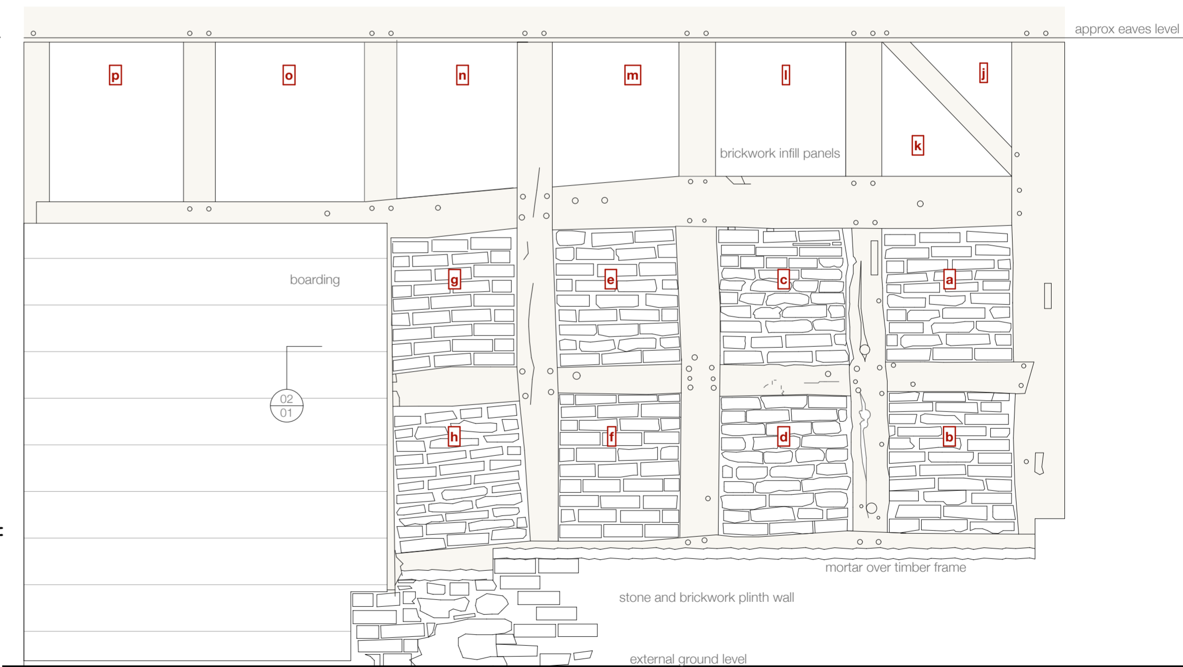
4. Timber Frame Exterior Elevation 1:20
