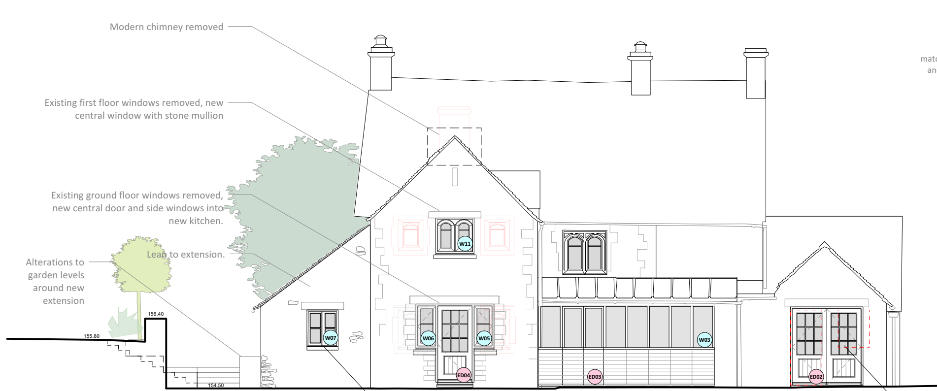
South West Elevation
