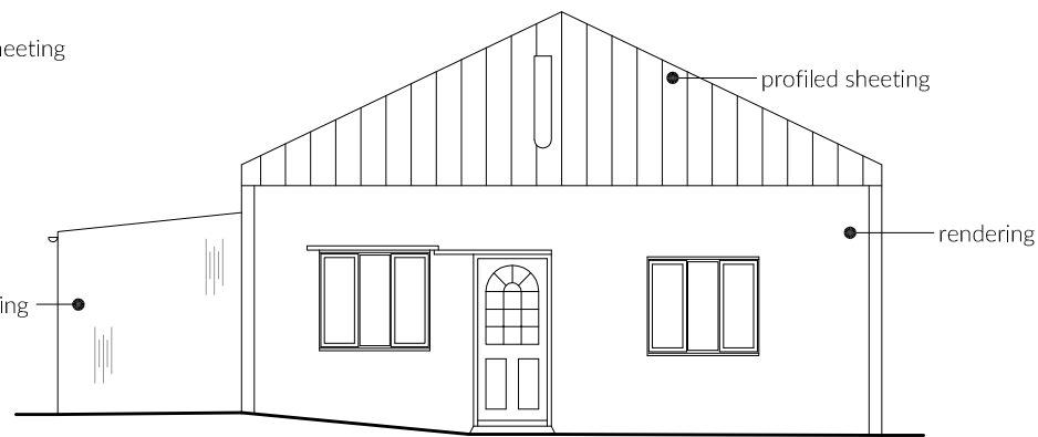
5 Existing South West Elevation 1:100
