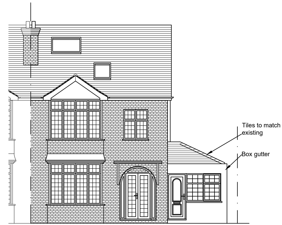
PROPOSED FRONT ELEVATION SCALE 1:100
