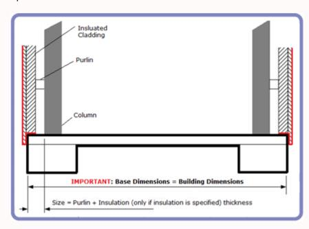
To ensure a weather we recommend creating a base that is raised off ground level by a minimum of 50mm to allow our cladding to overhang the base and promote water to run away from the structure. Our buildings can be erected to oversized bases/yards however this does introduce the need for an alternative method of creating a seal around the
