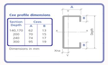
Cold rolled steel sections are incredibly strong for their weight. This means the combination of cold-rolled steel and portal frame methodology relatively small steel sections to span long distances.
