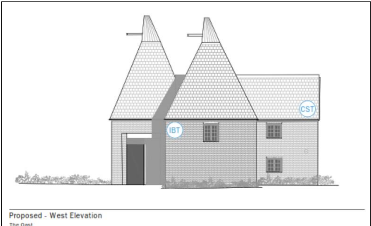
Figure A7.3: Proposed location for the crevice space tile (CST) on the western elevation on Building B2 to replace Roost 3 (common pipistrelle day roost used by one individual) and integrated bat tube (IBT) to replace Roost 4 (common pipistrelle day roost used by three individuals).
