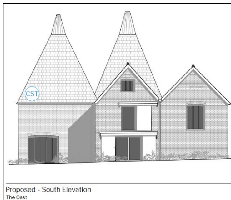
Figure A7.2: Proposed location for the crevice space tile (CST) on the southern elevation on Building B2 to replace Roost 2 (common pipistrelle day roost used by one individual).
