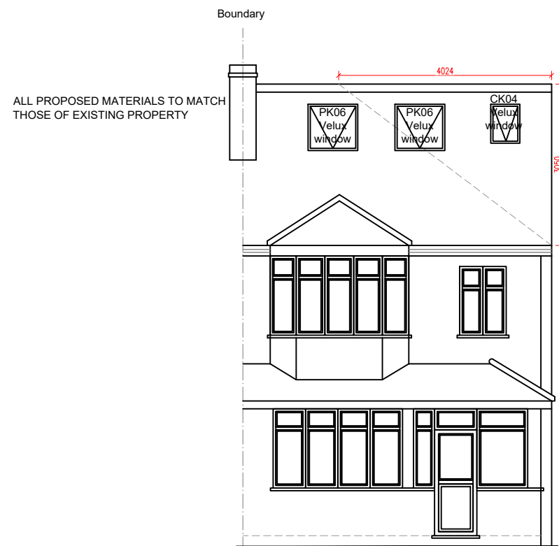
PROPOSED FRONT ELEVATION SCALE 1:100
