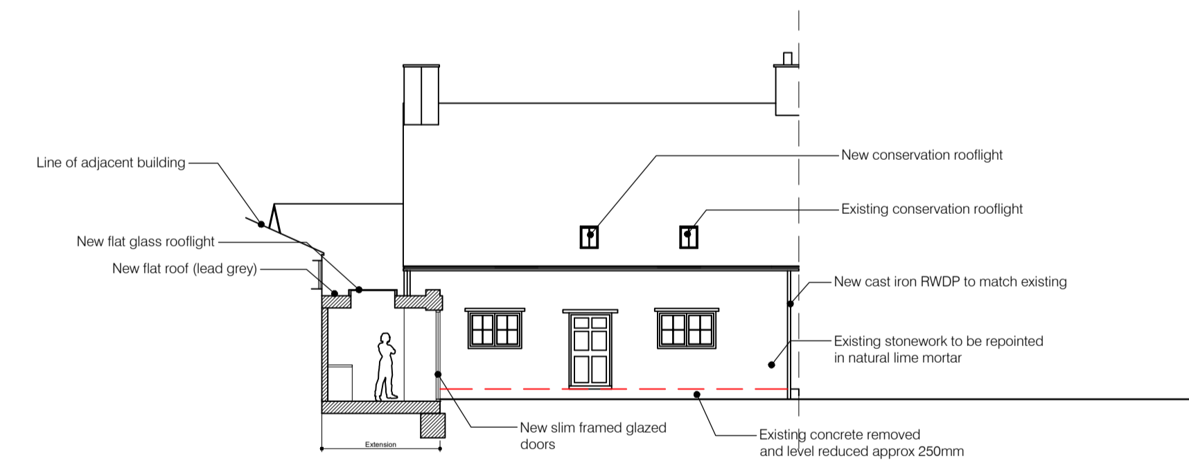
5 SOUTH WEST ELEVATION / SECTION A-301 SCALE 1:100 @A1
