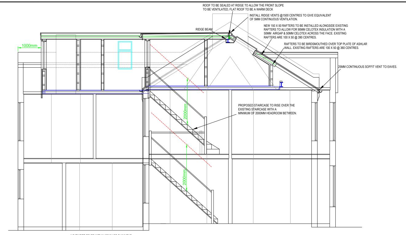
EXISTING JOISTS AND TRIMMERS TO FIRST FLOOR TO BE VERIFIED ON SITE FOR ADEQUACY TO CARRY ADDITIONAL LOADS. ESCAPE ROUTE AND CIRCULATION AREAS (INCLUDING STAIRCASES) TO BE CONSTRUCTED TO AT LEAST ½ HOUR FIRE RESISTANCE. WALLS TO BE SOLID OR IF STUDWORK, 2 LAYERS OF 12.5MM PLASTERBOARD TO BE PROVIDED OR VERIFIED ON SITE. LANDING TO BE OVERLAID WITH HARDBOARD IF NECESSARY. ANY GLAZING TO BE ½ HOUR FIRE RESISTANT.
