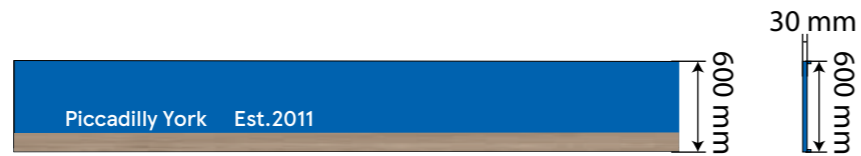
SIGN 1 4400x600 mm New non-illuminated timber fascia panel to be painted, Blue RAL 5005, 30% Gloss with Brown Arizona Oak woodtex strip to base. Store Address and Est. year vinyl lettering applied to new fascia. Ht: 100mm
