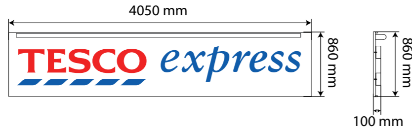
SIGN 2 4050x860 mm New pinned off externally illuminated Acrylic letters with 'Tesco' in opal 030 Avery 4509 Red 431, And Express & blips in Opal 030- Avery 5600 LD/082A blue acrylic letters fixed on timber panel.
