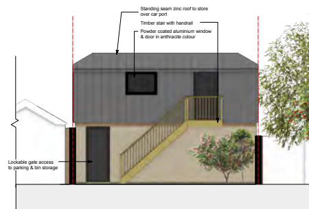
2 South East Elevation of Car Port Thro' Garden Scale: 1:50
