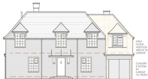
PROPOSED FRONT ELEVATION (SOUTH-WEST) 1:100
