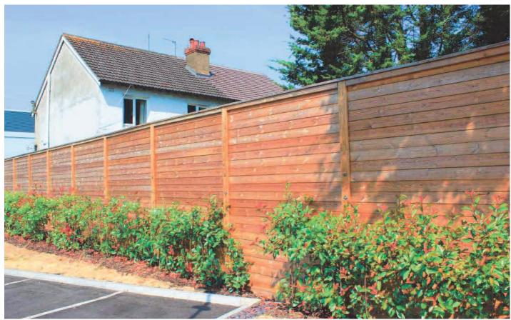
The Jakoustic<sup>®</sup> reflective barrier reflects the noise away using heavy section planed timber boards with a special profile that has been carefully developed. Boards are constructed in such a way that eliminates gaps that sound can easily travel through. Up to 28 dB\* in noise reduction.
