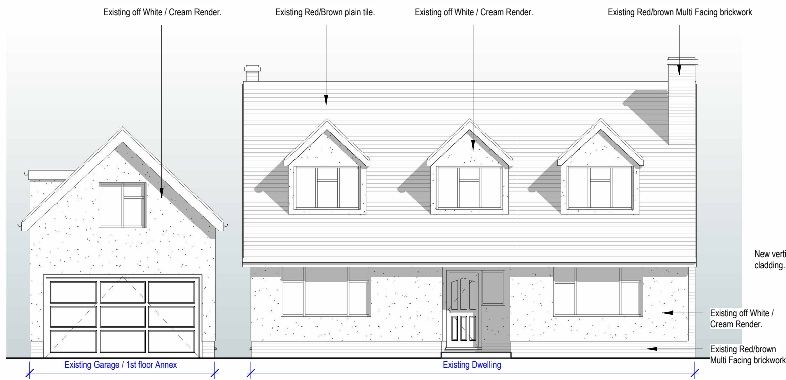
2 Existing Front Elevation. 1 : 100
