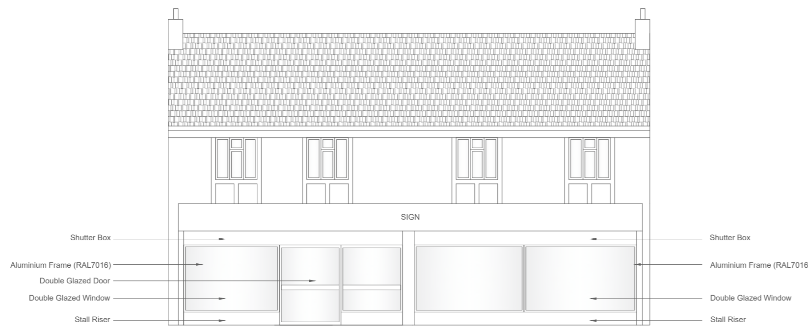
EXISTING FRONT ELEVATION
