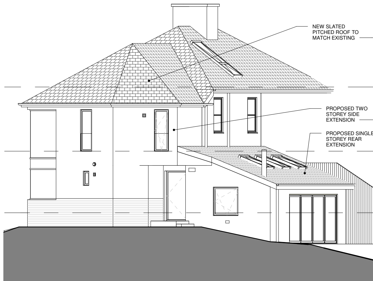
SIDE ELEVATION (E) AS PROPOSED @ 1:100
