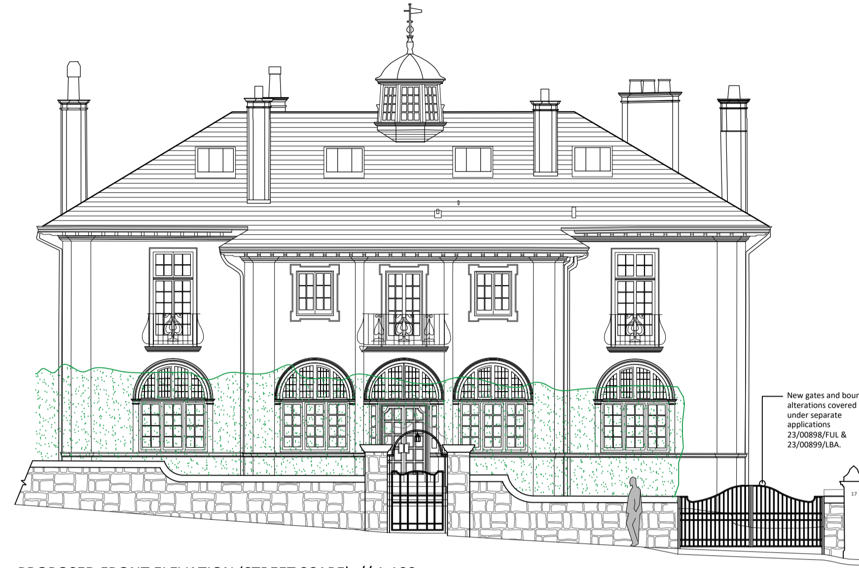
PROPOSED FRONT ELEVATION (STREET SCAPE) // 1:100
