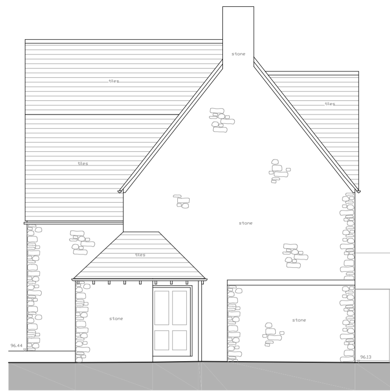
Existing Farmhouse East Elevation Scale 1:100
