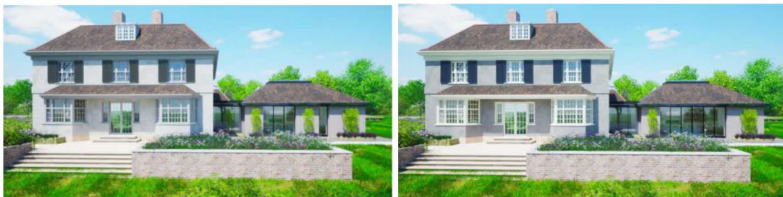
Fig.7&8 - Developed fenestration design to find the traditional/modern balance by reducing oversized glazing, introducing additional structure, and incorporating planting to ground the proposal. Preference for singular grouped doors, maintaining simplicity. Slight offset with a larger expanse of wall to the northern side, forming a bookend. The informality of the design contrasts the formality of the main house and responds to the subservient nature of the extension.
