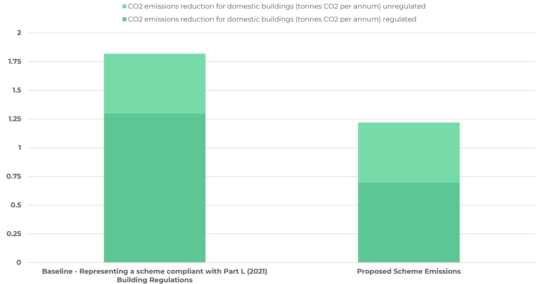
Figure 5: Total regulated carbon dioxide savings achieved through an energy efficient design and low carbon energy strategy.
