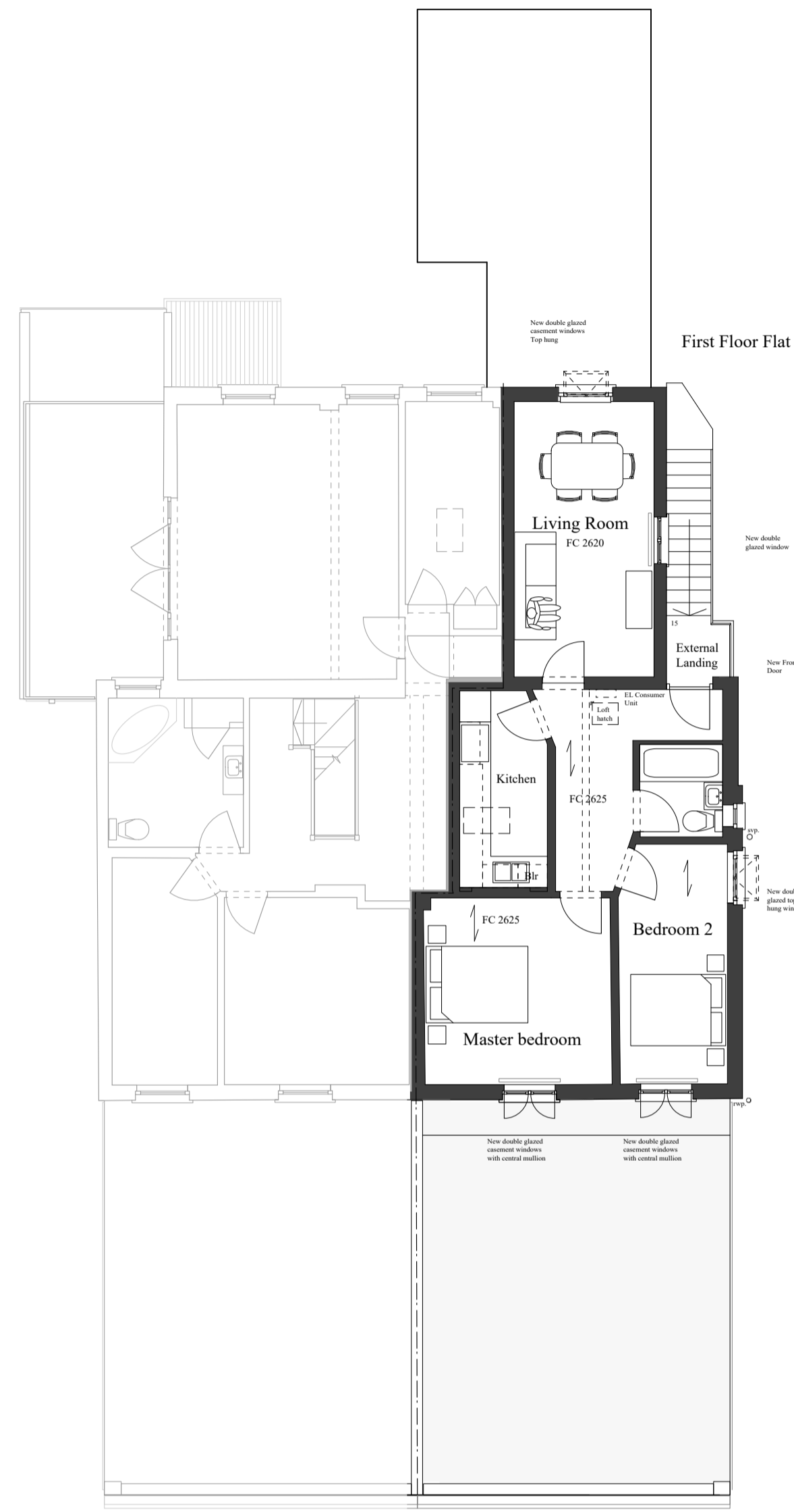
First Floor 2 Bed Flat Scale 1:100 @A1
