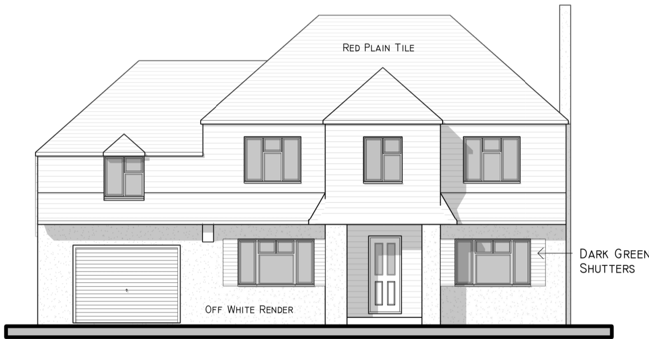
FRONT ELEVATION - EXISTING 1 : 100
