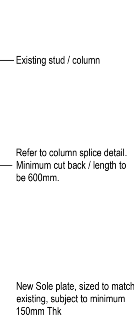
EAVES PLATE SPLICE DETAIL 1:10
