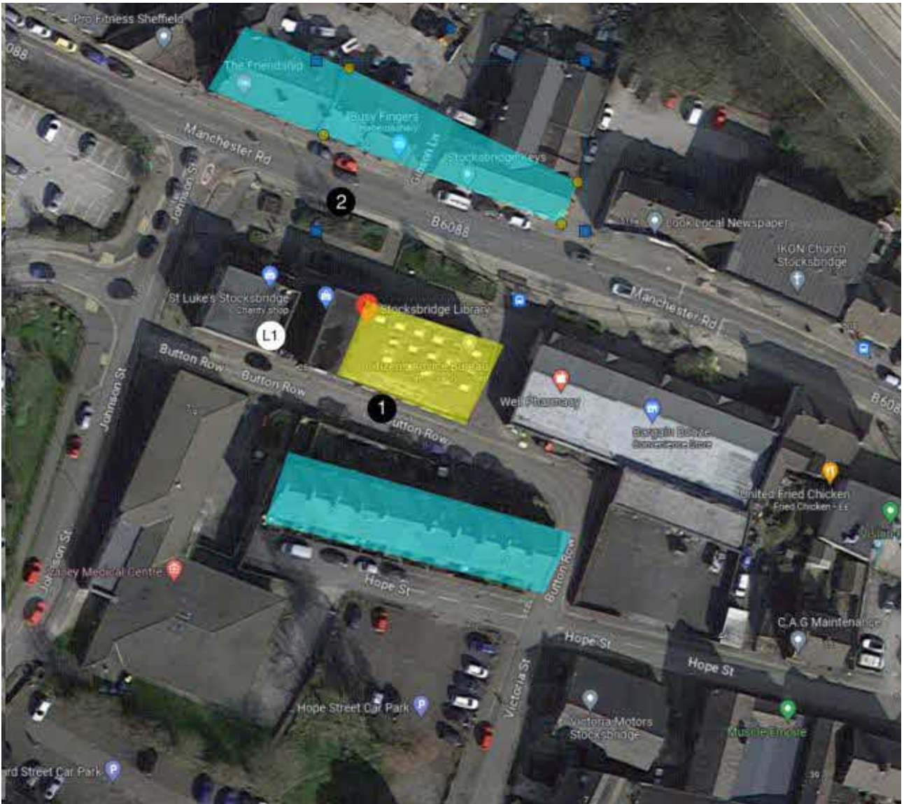
Figure B2.1 Image of site location with current library highlighted in yellow and the nearest noise sensitive receptors highlighted in blue. Measurement locations shown as circles (black circles show attended short-term measurement locations and the white circle shows unattended long-term measurement location).
