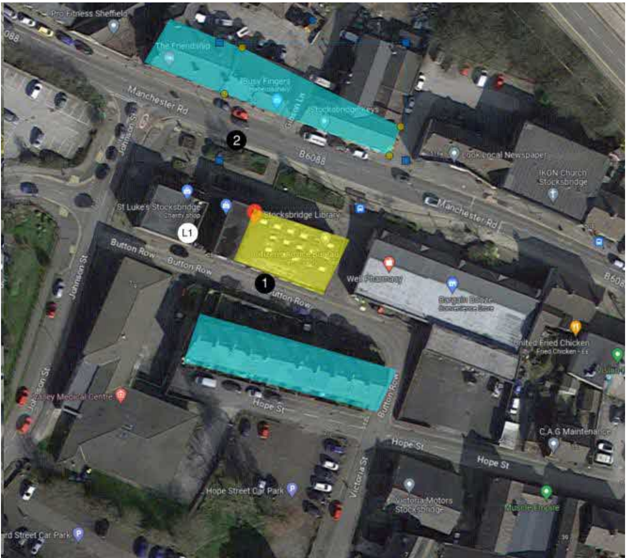
Figure 2 Measurement locations shown as circles (black circles show attended short-term measurement locations and the white circle shows unattended long-term measurement location); nearest noise sensitive receptors highlighted in blue; existing library highlighted in yellow.
