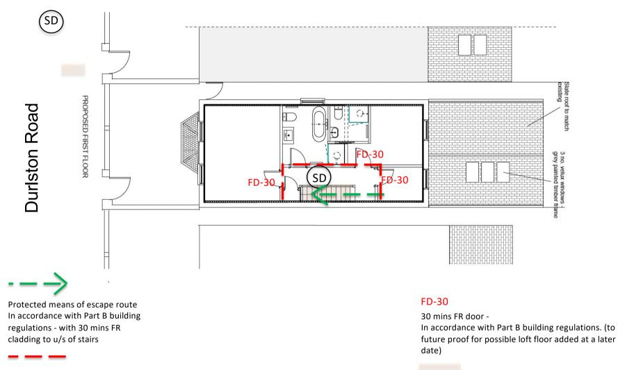
30 mins FR wall construction In accordance with Part B building regulations.
