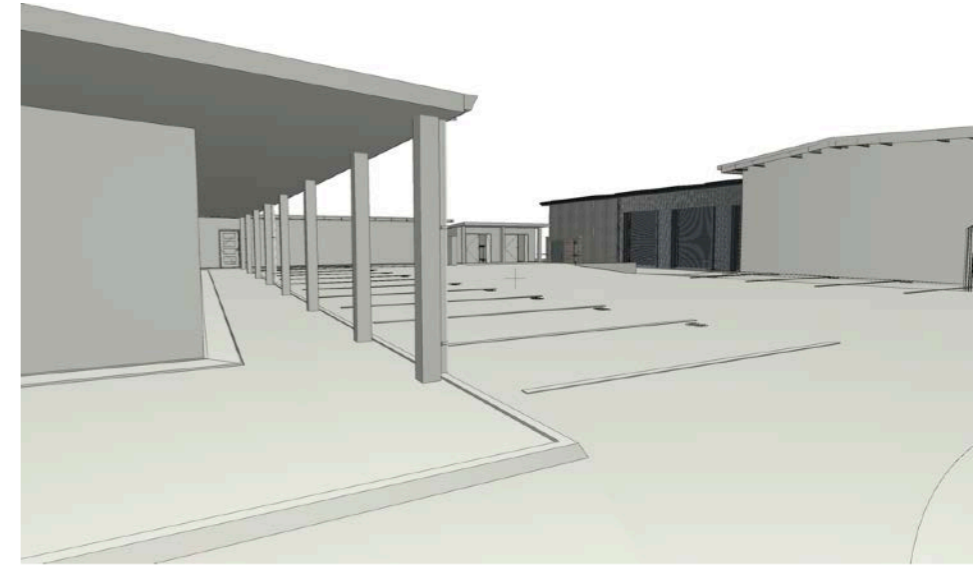
Courtyard view from rear of Wedding Venue servicing area. The finished floor level has been set below the level of the workshop and wedding venue to fall with the natural shape of the land and ensure the building appears sub - serving to the principal mass of wedding venue.
