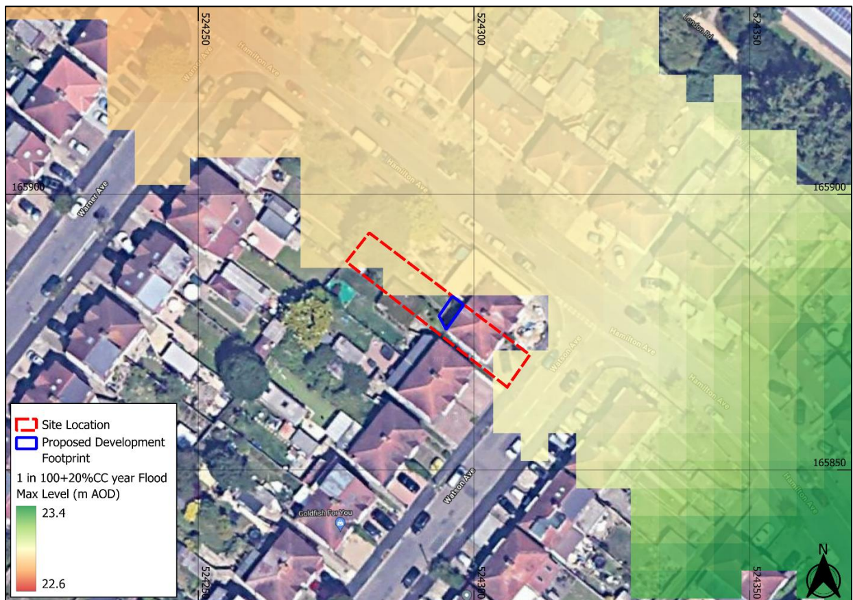
Figure 7: EA Modelled 1 in 100 plus Climate Change (20%) Flood Levels (Base map from Google Hybrid © Contains public sector information licensed under the Open Government license v3.0)
