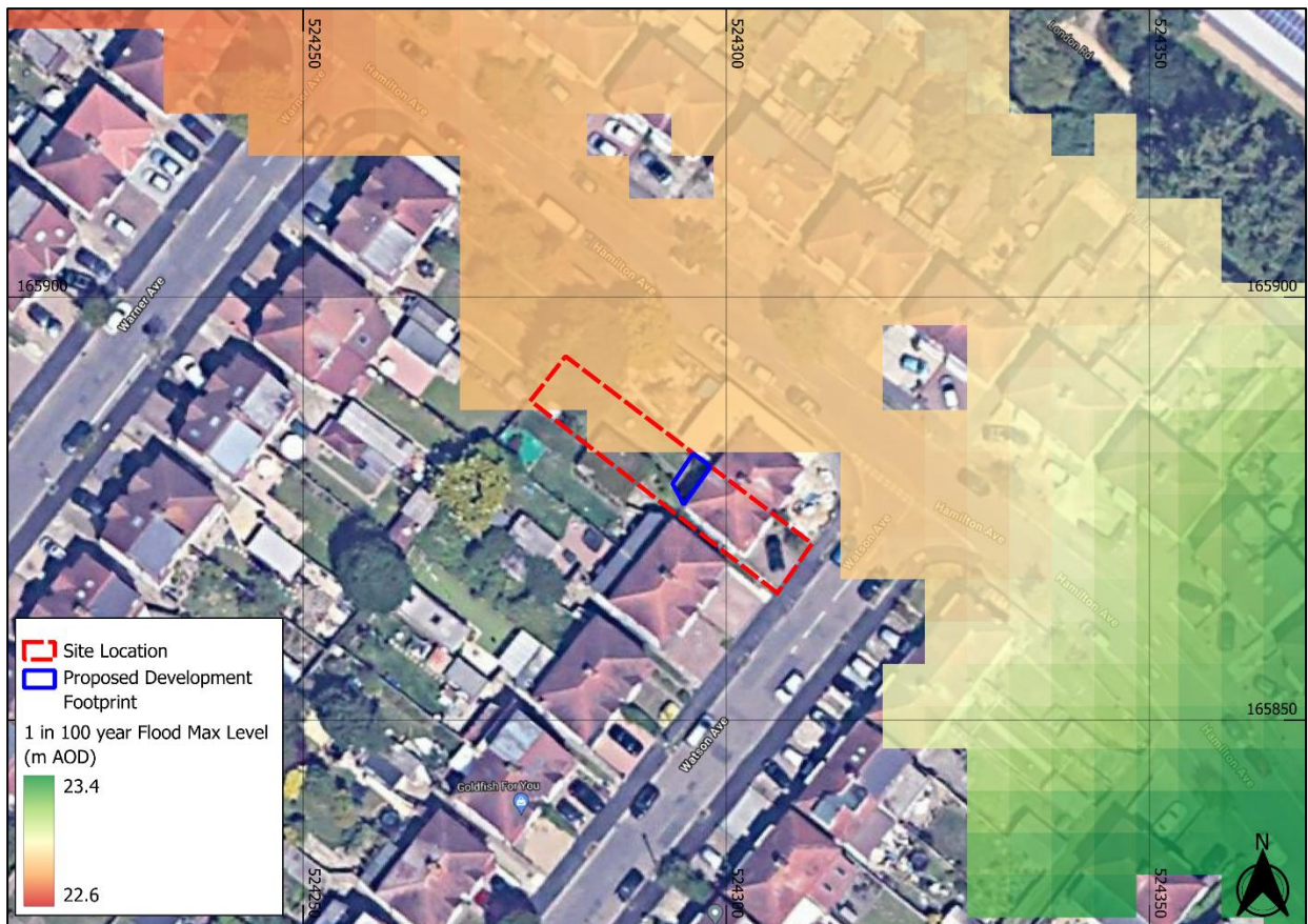
Figure 6: EA Modelled 1 in 100 Flood Levels (Base map from Google Hybrid © Contains public sector information licensed under the Open Government license v3.0)
