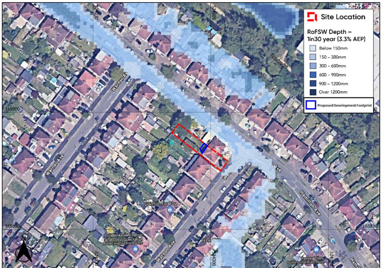
Figure 9: EA Surface Water Flood Risk Mapping 1 in 30 Year Depth (Base map from Google Hybrid © Contains public sector information licensed under the Open Government Licence v3.0)
