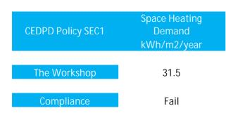
The ultimate goal is to reduce the total energy demand of the proposed development. In this instance the total space heating demand is marginally higher than the 30 kWh/m2/year and so the scheme technically fails to comply with the Councils requirement on this individual aspect, however the non compliant heating demand does not prevent the building from being low energy use and achieving the net zero carbon threshold.
