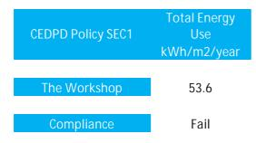
As the results are more than 40 kWh/m2/year then the scheme fails to comply with the Councils requirement.
