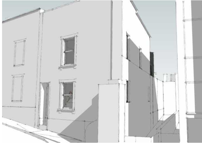
Photo 16. View of the restored front elevation with new painted timber sash windows, door and stone surrounds. The proposed windows on the side elevation can also be glimpsed in the narrow space between the application property and no. 1 Old School Lane.
