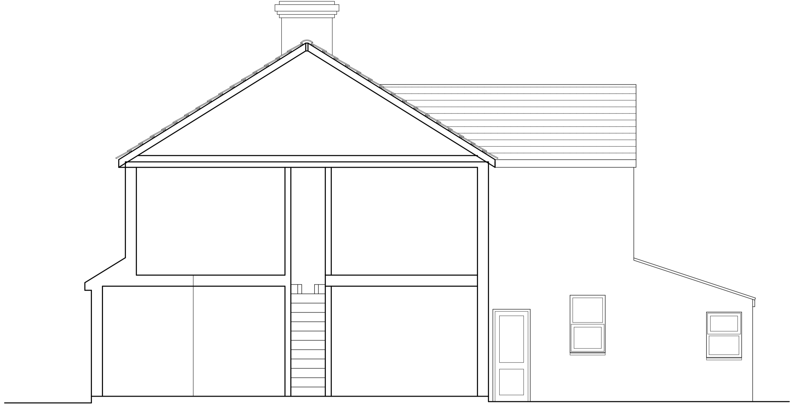
EXISTING SECTION/SIDE ELEVATION
