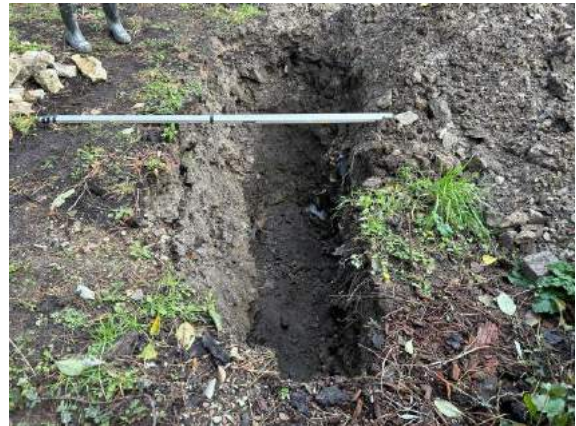
Photo 10: TP01 Test 2 completed (9 mins 42 secs) from Face B looking 250 W
