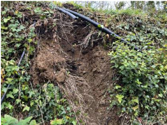
Photo 13: Prior cut to the east showing Topsoil over Residual Soil looking E
