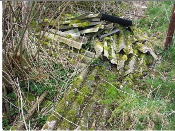
Photo 16: Corrugated cement/asbestos sheeting
