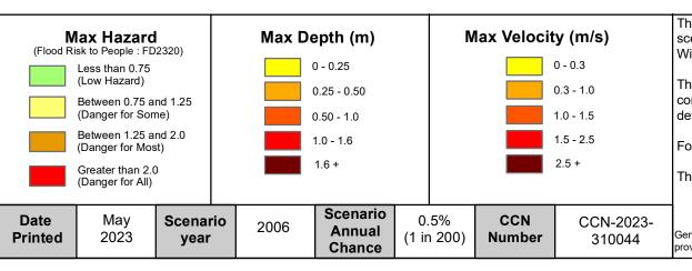
The map is based on computer modelling of simulated overtopping of the main coastal defences for specific tidal scenarios. It does not include overtopping along the following tidal rivers which are currently being investigated: Witham Haven (upstream of Hobhole), and Welland (upstream of Fosdyke Bridge)
