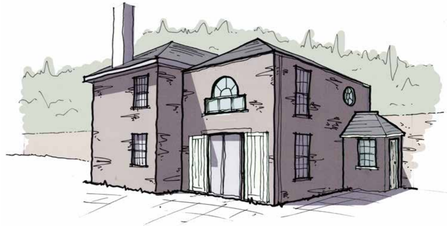
FINAL DESIGN - SIDE PORCH ADDED TO EAST (REAR) ELEVATION, NEW WINDOWS ON SOUTH ELEVATION OF EXTENSION ECHOING DESIGN OF NEARBY STABLE BLOCK
