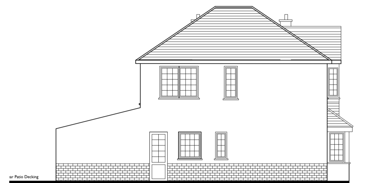
Existing West Elevation
